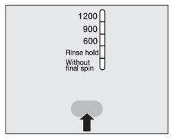
■ Press the "Spin" button enough times until the indicator light for the required final spin speed lights up.
